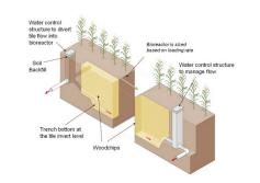
Denitrifying Bioreactors are essentially subsurface trenches filled with a carbon source, mainly wood chips, through which water is allowed to flow just before leaving the drain to enter a surface water body. The carbon source in the trench serves as a substrate for bacteria that break down the nitrate through DE nitrification or other biochemical processes. Bioreactors provide many advantages:
